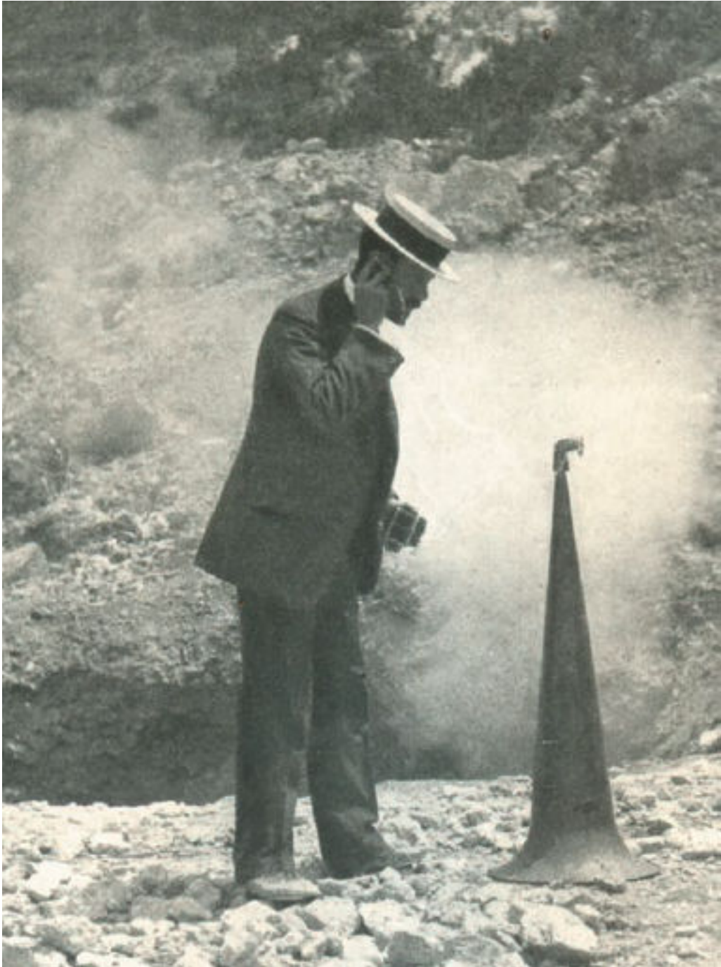
F. A. Perret with an improvised “geophone,” listening to subterranean noises at the Campi Flegrei, Italy, c. 1906-1907. Source: “The Day’s Work of a Volcanologist.” The World’s Work , V. 25, November, 1907.
